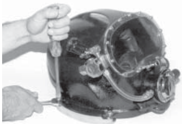
Adjust Cams with a wrench and screwdriver.
