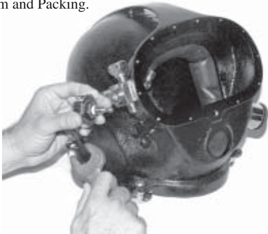
Remove the Valve Stem and Packing from the Manifold Body.
