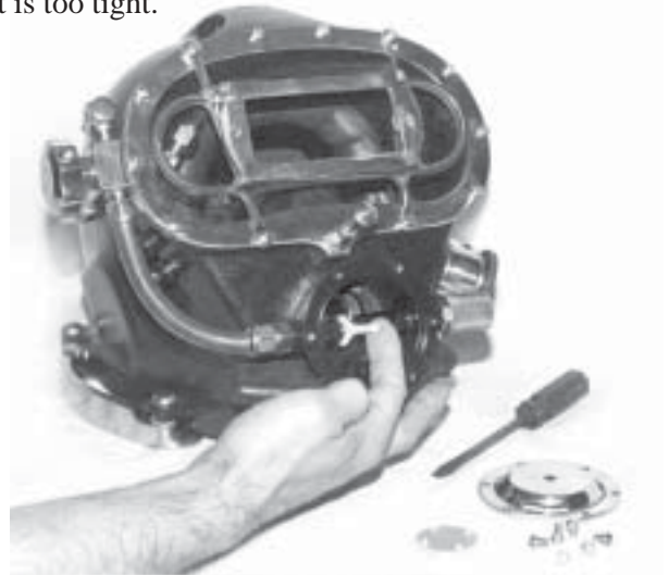
Check Free Movement and position of Lever (88).
